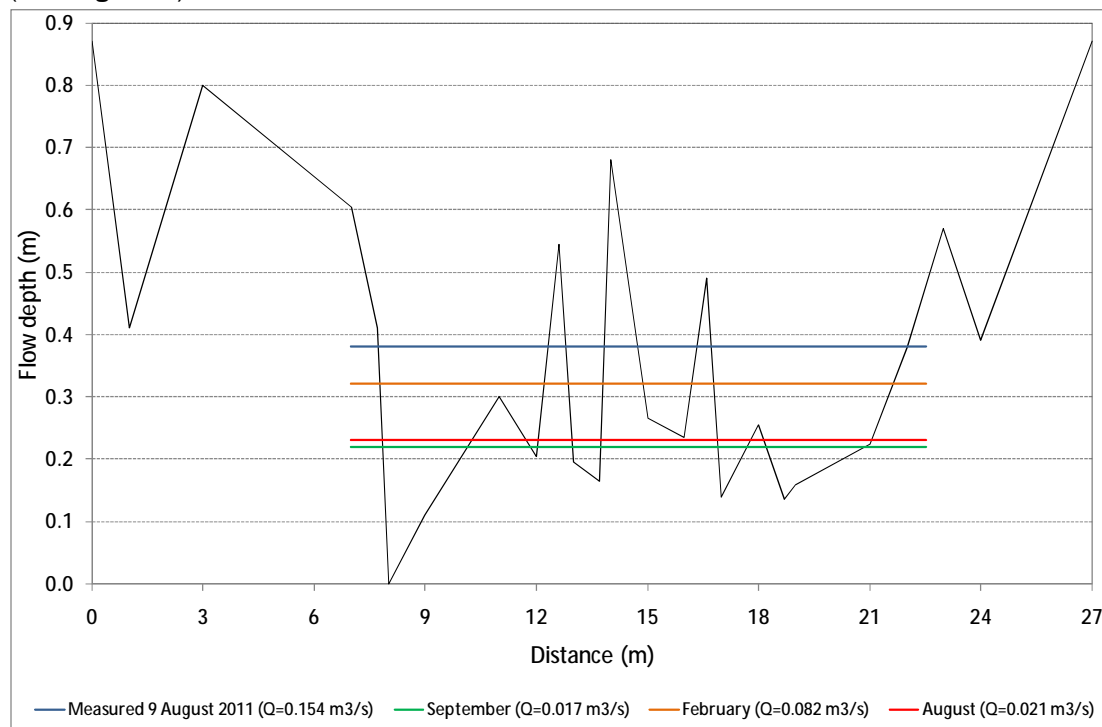
Figure 7: Calibrated cross-sectional profile of the Kranspoortspruit at the EWR site
